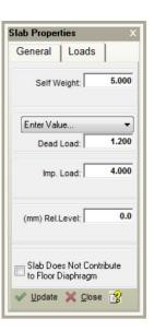
Orion calculates the self-weight of the slab automatically from its thickness and the concrete density (specified earlier when defining materials).
